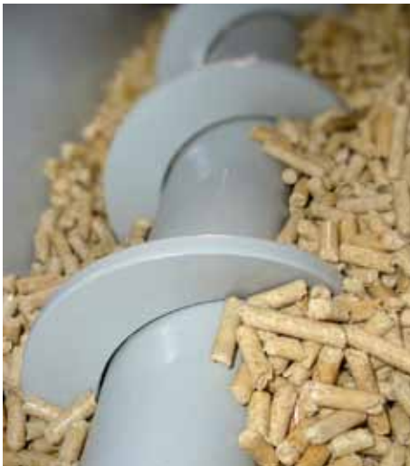
The HDG pellet delivery worm conveys pellets from rectangular storage rooms.
