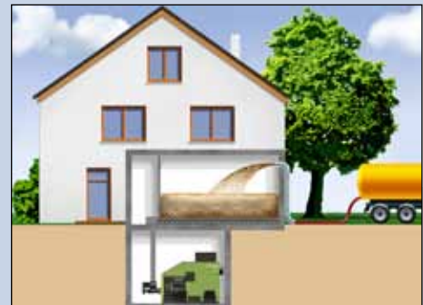
Example: pellet bunker in cellar with blower system
