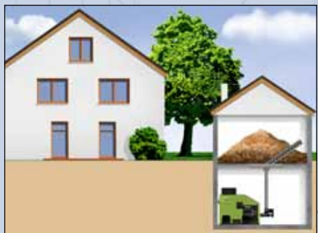
Example: silo delivery from a chip silo using a silo feeding system
