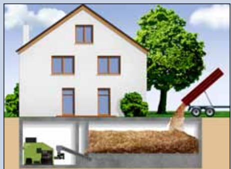
Example: walking floor feeding system with filling via a load-bearing ceiling
